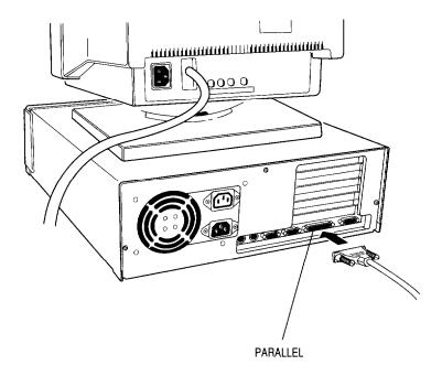
3. Connect the other end of the cable to the printer as shown below. To secure the cable, squeeze the clips at each side of the printer port and push them into place.
